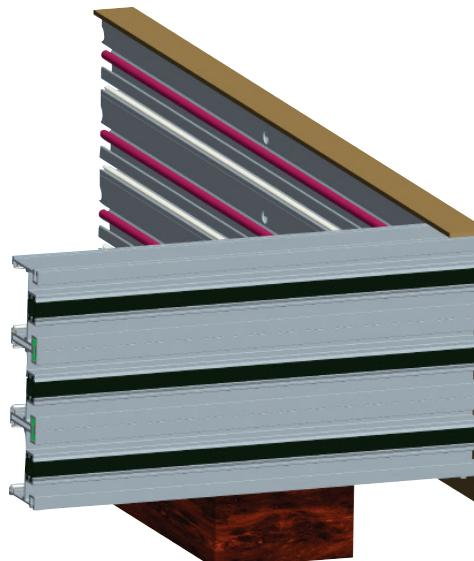
Drill holes onto L shaped panel based on pre-drilled holes on the door sill.
