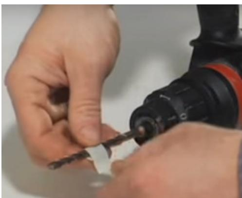
Use masking tape to mark 2" on the drill bit as shown in the picture this will help reach the desired depth on the concrete.
